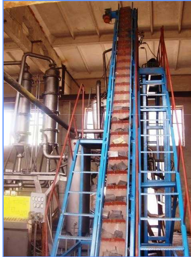
Conveyor for raw material submission.
